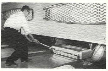
Special, adjustable handle lowers to permit complete cleaning of the pin deck. The machine is purposely designed with a low silhouette to assure sufficient headroom clearance.
