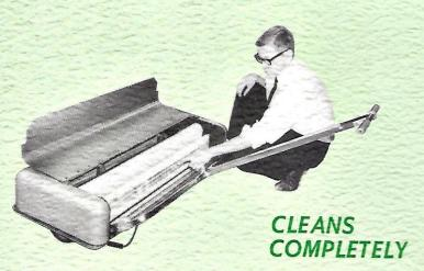
With the Lino-Matic, dust is always picked up, never pushed along. Pines "Red Edge" cloth is held to the lane by a sponge-type roller and is advanced continuously, automatically to assure that clean cloth is always in contact with the lane. Larry Unterbrink points to a three lane pattern of dust pick-up. Note: the dust is not just in one thin line across the cloth, but covers at least one inch per lane. Even pick-up like this assures uniform cleaning at minimum cost.
